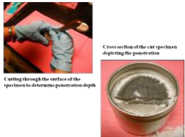
Figure 11 Penetration test for prime coat
